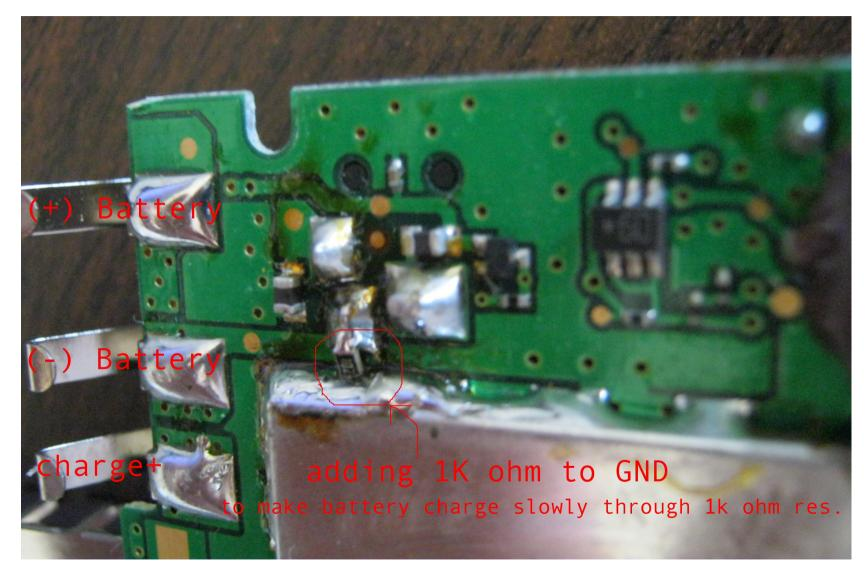
to isolate normal charging build in radio, it need to cut out parts of terminal in Yellow Battery Case. to make it same as Black Case.
