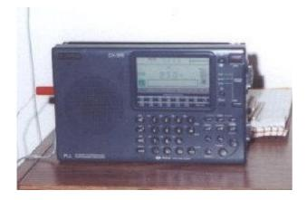
initially this radio in U.S. come with FM frequency coverage of 87.5 - 108 MHz, it can be modified to cover such as Japanese or Eastern Europe FM frequency.
