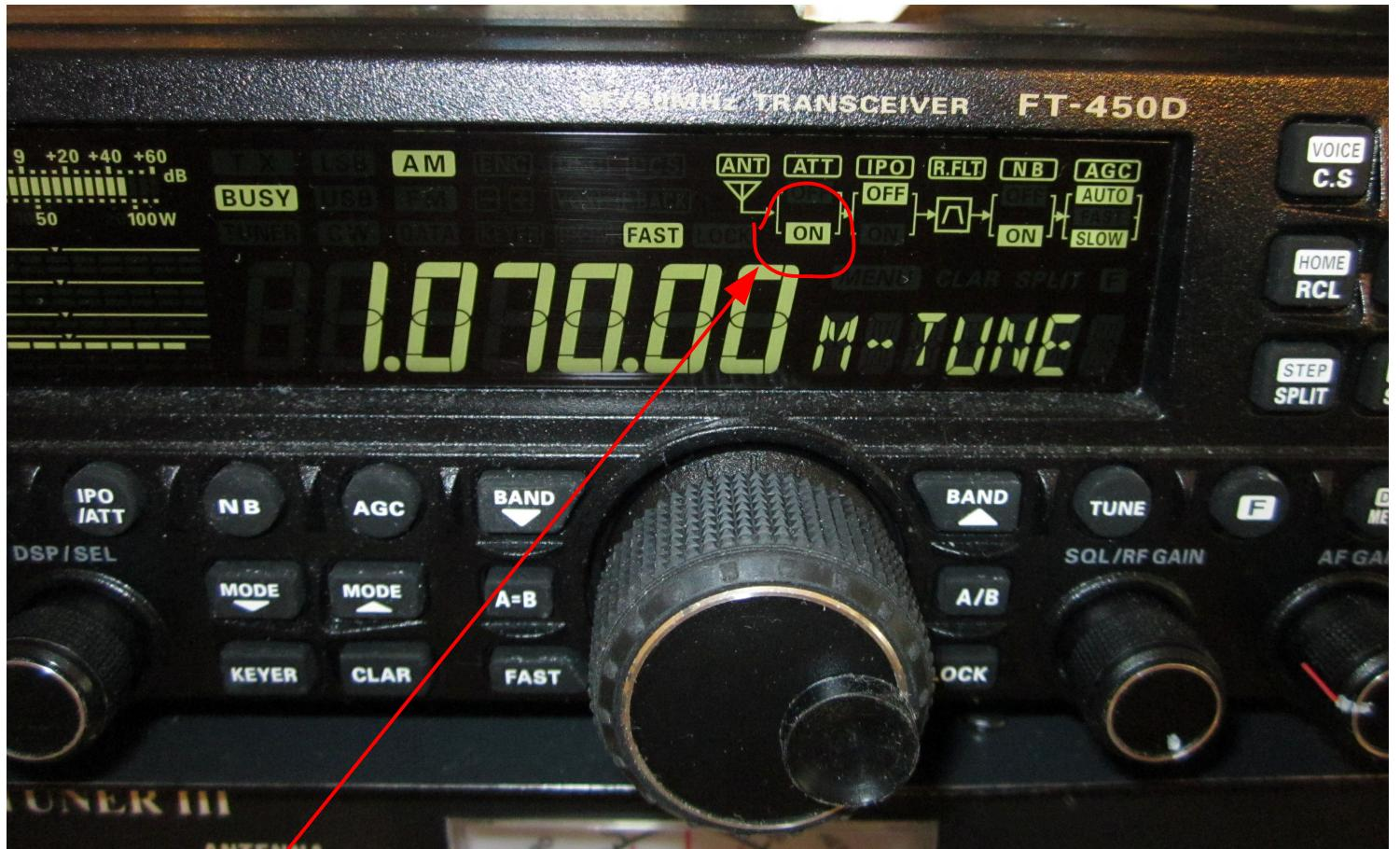
at frequency below 1700kHz, even the display say ATT is ON,
